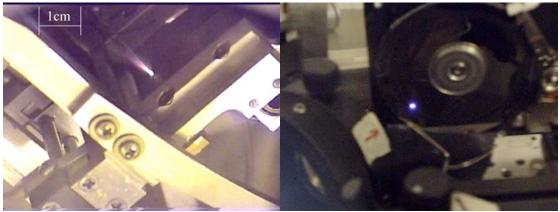
**Figure 4. Jets from the ms-pulse (left) and ns-pulse microthrusters** in vacuum [see, e.g., 12]. The ns-pulse jet was demonstrated in tests with a spinning laptop hard drive diskk, and operated for 4 hours.
